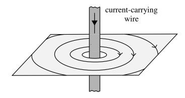
(ii) current in one turn produces magnetic field in region of adjacent turn; this gives rise to force in adjacent turn which also has electric current; they attract;
